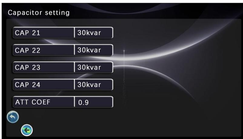
Capacitance setting: Set the compensation capacity of each circuit according to the actual system configuration, with a range of 0-900kvar.
