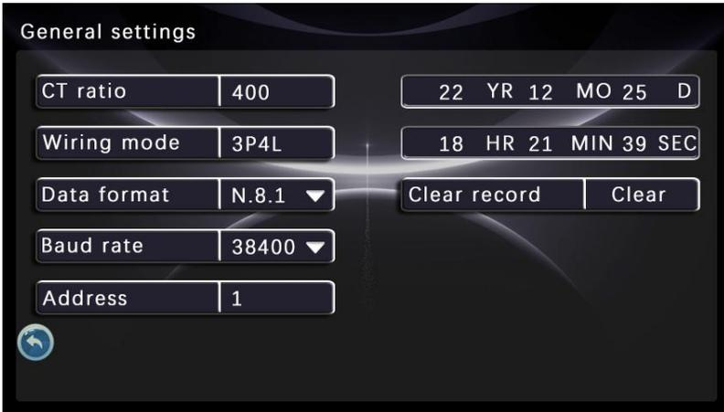
External transformer ratio, wiring method, time, and event reset can be set. Set communication parameters, one communication line can be set, with instrument address range of 1-247 and baud rate of 480096001920038400; The data formats are N81, N82, E81, and O81 (with no parity, even parity, and odd parity, respectively), and the communication protocol is standard Modbus-RTU. The communication address table is shown in the appendix.
