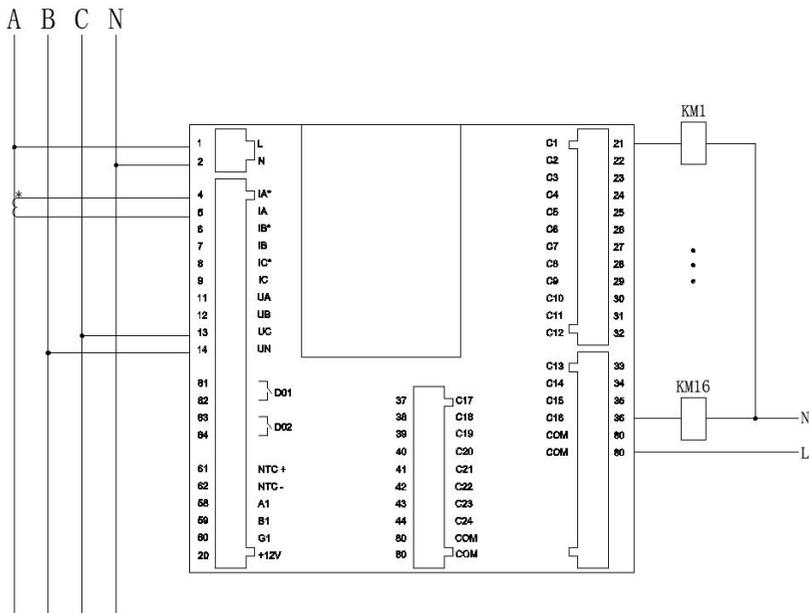
Total compensation (1P2W)Static wiring diagram
