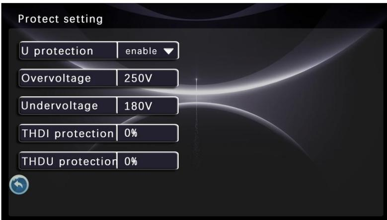
Two types of protection can be enabled or disabled, one is voltage protection, and the other is harmonic protection. Voltage protection is divided into undervoltage protection and overvoltage protection, while harmonic protection is divided into harmonic voltage protection (THDu%) and harmonic current protection (THDi%).
