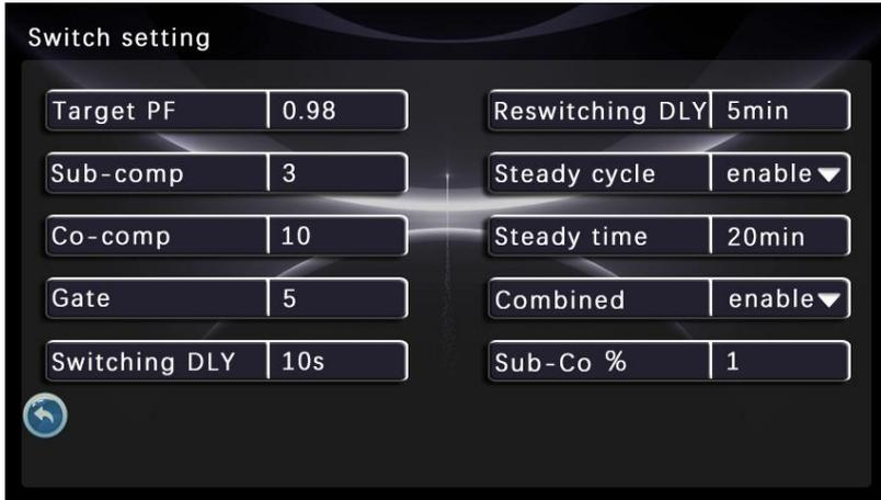
Target power factor: refers to the setting of the target power factor, with a value range of 0.500 to 1.000;
