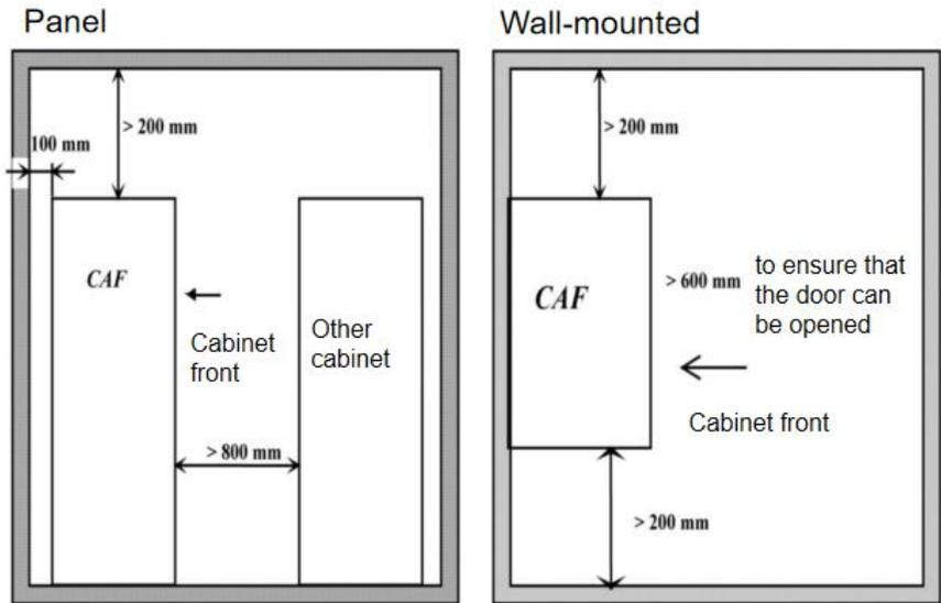
Figure 3-1 Device installation diagram
